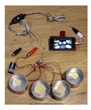
With a bit of luck, you can plug it straight in to a MIDI drum synth and start playing. The four pads transmit kick drum, snare, closed hi-hat and open hi-hat note values according to the General Midi specification (see "General MIDI Level 1 Percussion Key Map" at https://www.midi.org/specifications/item/gm-level... (https://www.midi.org/specifications/item/gm-level-1-sound-set)).
