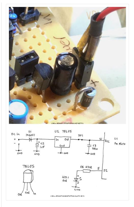
You can power the Arduino over its USB connection, plugging it in to a computer or a power bank. For maximum portability, though, I added a simple voltage regulator to run it from a 9V (PP3) battery. Current drain is about 50mA, so if you're going to use it a lot a rechargeable PP3 is a good idea. I included a removable jumper (JP1) so the regulator circuit can be disconnected when the Arduino is being powered from USB during programming.
