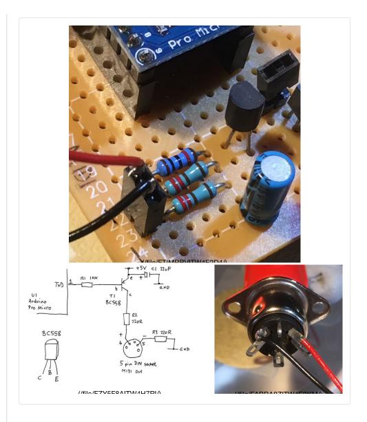
This bit of the circuit uses a transistor connected to the TXD (serial output) from the Arduino to drive the MIDI output, as shown in the circuit. Make sure you get the C, B and E connections on the transistor the right way round - the BC558 and many other transistors are connected as shown in the sketch, but some other types can vary.
