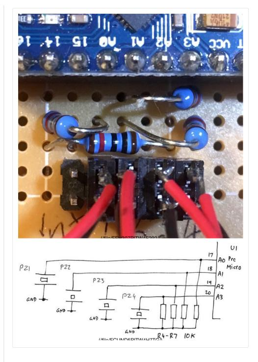
Each pad is connected directly to one of the Arduino's analog inputs (A0-A3), with a 10K resistor connected to ground as shown. You'll need a connector of some sort to allow the pads to be unplugged while assembling the rest of the board.
